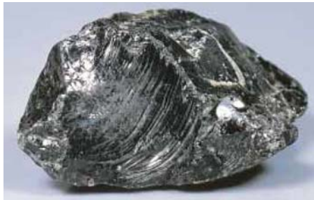
Figure 5–1. Quartz typically fractures along smoothly curved surfaces, called conchoidal fractures. This sample is smoky quartz.
